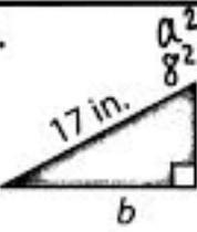
$\begin{aligned} a^2 + b^2 &= c^2 \\ 8^2 + b^2 &= 17^2 \\ 64 + b^2 &= 289 \\ b &= 15 \text{ in.} \end{aligned}$                                                                                |
